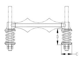
MATERIAL: Spring cushion hanger is composed of a set of two springs and four cast iron retainers.
