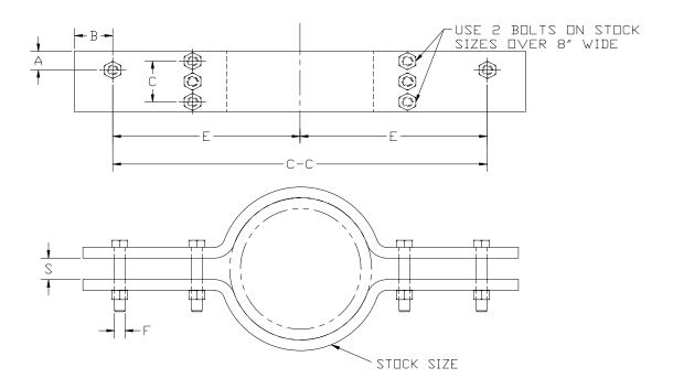
MATERIAL TYPES: Carbon steel, chrome molybdenum or stainless steel.
